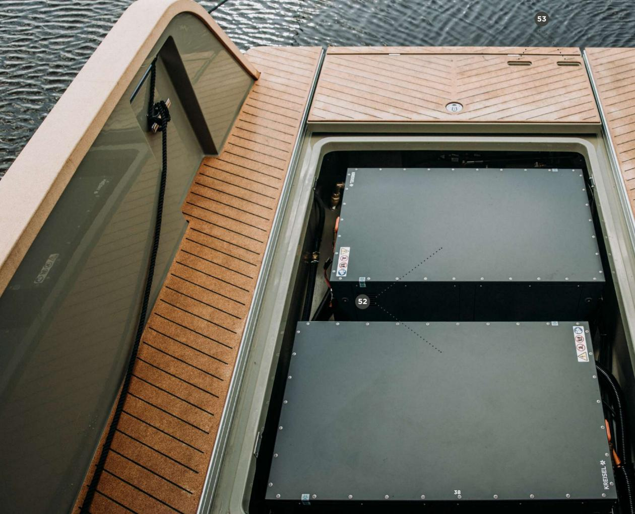
52 120 KWH LIQUID COOLED IP 67 LITHIUM ION BATTERIES (2 X 60KWH)
