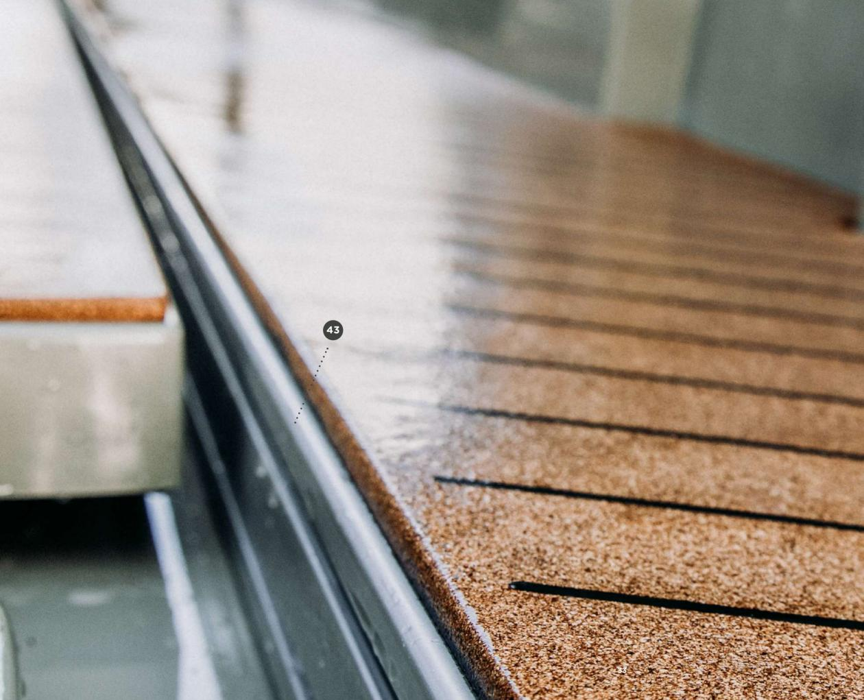
43 19 FEET ALUMINIUM RAILS TO LOCK MODULAR INTERIOR TO THE DECK
